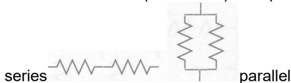
*In series circuits, the DC current is the same through all of the components (what goes in one end equals what comes out of the other end). In parallel circuits, the voltage is the same across all components.*
