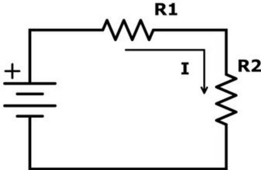
Figure 3. A series circuit.
